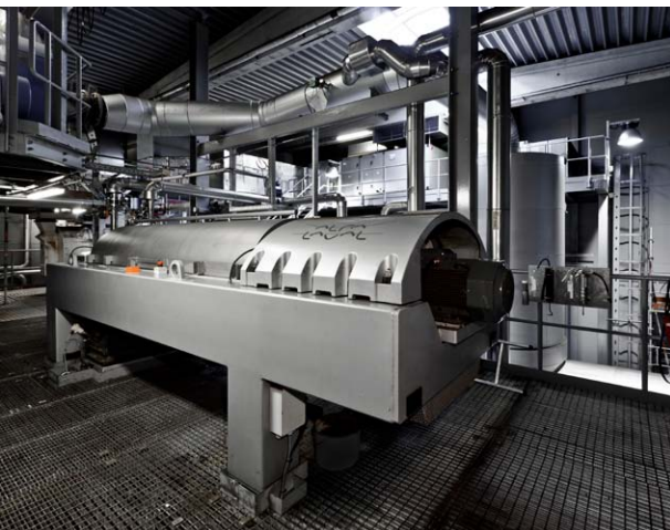
Alfa Laval decanter centrifuges are characterized by high separation efficiency, low power consumption, high capacity and easy handling.
